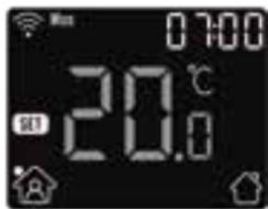
On the actual temp page, Press the up-key and down-key to set temporary override temp. The temp is only valid at the current event and it will not be saved.
